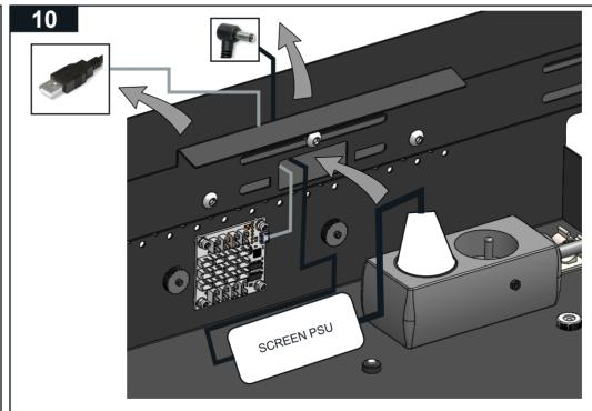
FEED BOTH THE SCREEN POWER CONNECTOR AND USB THROUGH THIS HOLE AND OUT THE TOP OF THE REAR CHANNEL.
