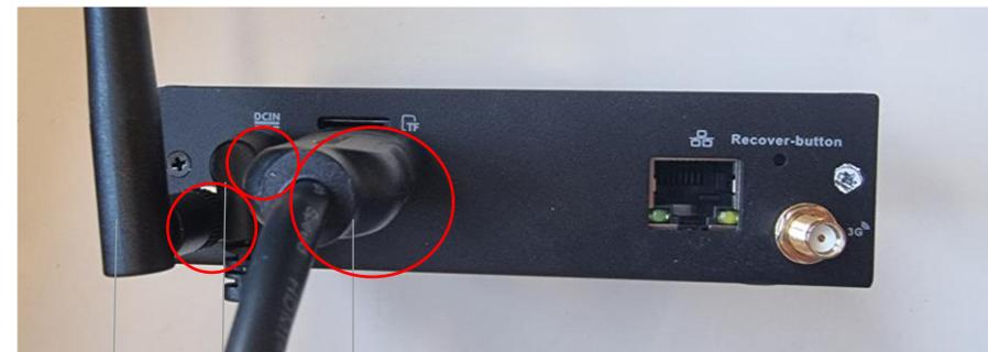
Wi-Fi Antenna Power Lead HDMI
