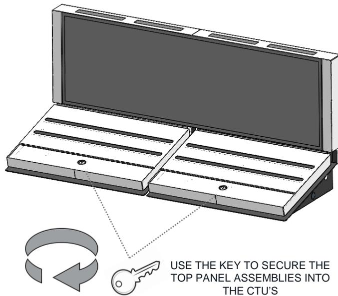
USE THE KEY TO SECURE THE TOP PANEL ASSEMBLIES INTO THE CTU'S
