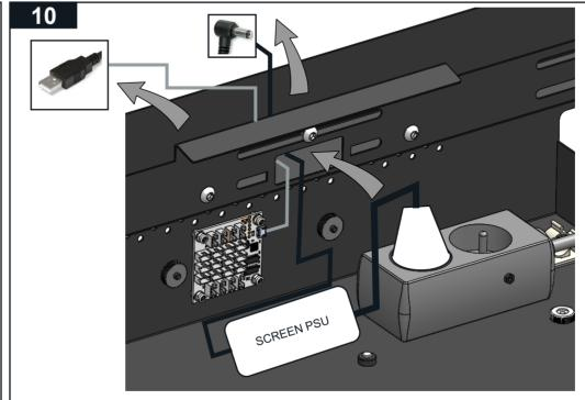
FEED BOTH THE SCREEN POWER CONNECTOR AND USB THROUGH THIS HOLE AND OUT THE TOP OF THE REAR CHANNEL.
