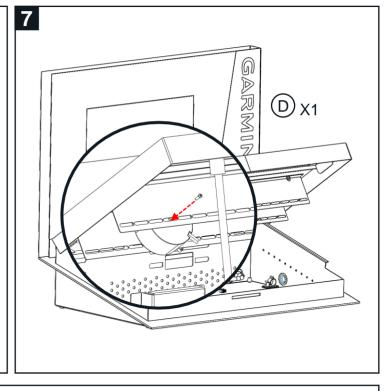
CLIP RJ9(1) CONNECTOR INTO SOCKET IN TOP MOULDING
