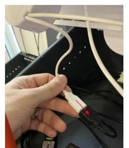
Connect USB from pull box to USB splitter in base.
