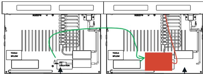
PLU MEDIA PLAYER PSU INTO 1<sup>ST</sup> CTU TO POWER THE MEDIA PLAYER. LOOM THE CABLE THROUGH GROMMETS IN THE SIDE OF THE METAL BASE.
