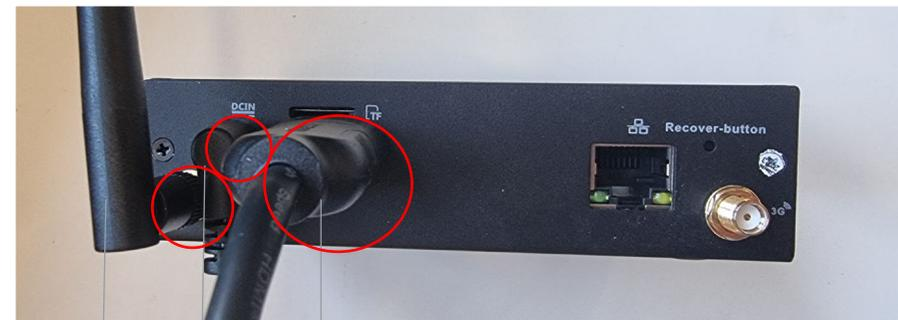
Wi-Fi Antenna Power Lead HDMI
