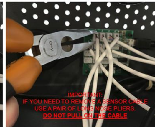
ENSURE THE SENSOR CABLE FROM SECURITY DEVICE 1 IS PLUGGED INTO PORT 1 ON THE PCB, AND SO ON FOR THE OTHER SECURITY DEVICES
