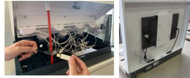
Insert USB into port inside base of unit or side of screen
