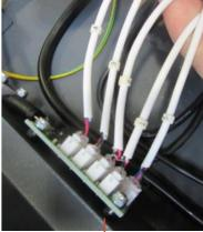
Lift and Learn cables for PCB board numbered 1-5
