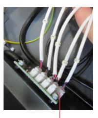
Lift and Learn cables for PCB board numbered 1-5
