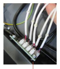
Lift and Learn cables for PCB board numbered 1-7
