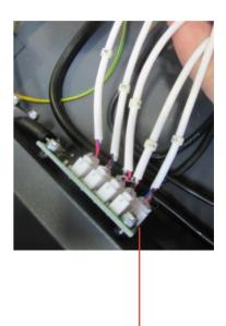
Lift and Learn cables for PCB board numbered 1-7
