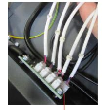
Lift and Learn cables for PCB board numbered 1-7
