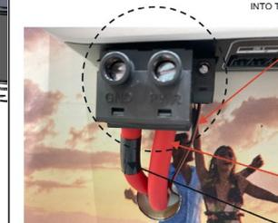
WIRE THE RED AND BLACK CABLE ITS THIS TERMINAL BLOCK ON AMP
