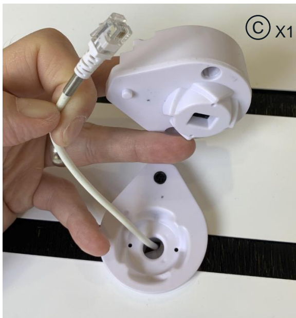
CLIP RJ9(1) CONNECTOR INTO SOCKET IN TOP MOULDING
