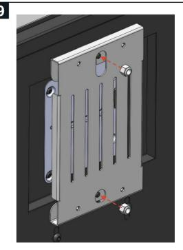
SECURE BRACKET WITH 2 OFF M6 LOCKING NUTS
